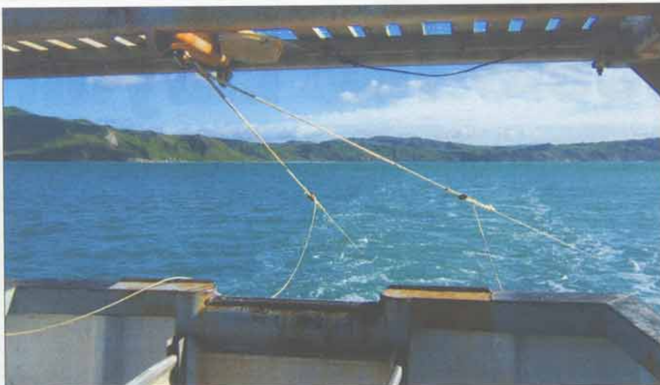
Above: Nancy Glen has no wire on board and the only chains are short lengths in top bridles to make adjustments easier. Even the donkeys the trawl is towed off are made from lengths of Dynex.
