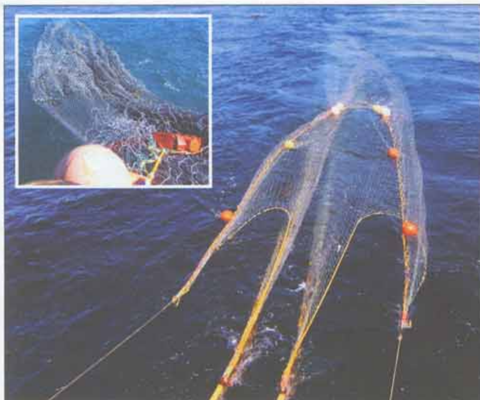
The T90 trawl after being re-cut with a taper. Only a few floats are needed to keep the gear square. Just six 6 in. floats and two 9 in. floats are needed. Inset: the T90 trawl in its original configuration before being re-cut.
